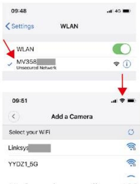
(4) Open the surveillance APP V380 Pro, scroll down the screen to refresh, then you will be able to see the new connected camera, click on the screen to set user name and password (like the picture shown below), if don't set the Password and Username (if need), the Short and Long range settings won't succeed. After setting successfully, you can watch the video from your phone.
