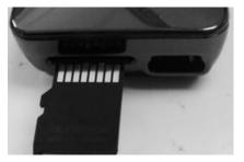
After the installing, please select the card inserting menu if you want to use TF card. Pressing down the card under turned off condition, it will pop out automatically.
