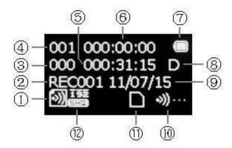
Bluetooth mode (2)Serial number of current file (3)Total files (4)The number of current file (5)Total time of surplus recording files (6)Time of current recording file (7)Electric quantity (8)Recording files folder (9) Date of file (10)Bluetooth record (10)Storage menu (10)Record type
