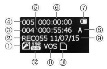
①Record mode ②Serial number of file ③Total files ④The number of current file ⑤Total time of surplus recording files ⑥Time of current recording file ⑦Electric quantity ⑧Recording files folder ⑨Date of file ⑩Menu of storage ⑪Identification of VAR ⑫ record type
