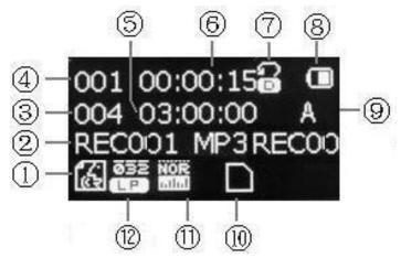
(1) Voice mode ②Serial number of current file and display ③Total files ④ The number of current file ⑤Total time of current recording files ⑥Time of current recording file ⑦Circulate mode ⑧Electric quantity ⑨Recording files folder ⑩Display menu ⑩Sound effect mode ⑫Current record mode
