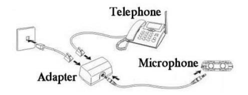
Connect the telephone under the turn off condition as the picture displaying, and then turn on the recorder start recording.
