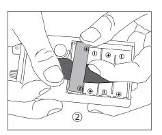
2.You can see a plastic band inside of the battery box. Place 4pcs of AAA battery over this band. You can pull up this band when you remve batteries. After you placing battery, put back the lid of battery box.
