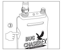
6.Press scan botton (③). BC-EX starts scanning giving off the "Pi..Pi..." sound. Right at this moment, BC-EX is scanning radio signal.
