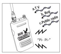
7.When BC-EX receive signal while scanning, it sends a discriminating tone (Pi- Pi- Pi-). At this stage, BC-EX telling you there's suspicious radio signal in the room. Keep holding BC-EX and keep the speaker facing forward.
