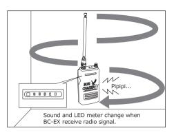
3.Hold BC-EX in your hand and move it like you wiping the wall or faniture. When BC-EX receives raido signal, it gives you an arart by changing the sound and LED meter. You cannot judge it is coming from bugging device right away even if BC-EX shows response. Check the area BC-EX shown the response with your eyes.
