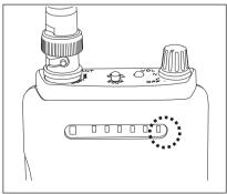
10. While BC-EX is running audio mode it stops receiving signal if the raido signal is too weak. When it stops receiving, the LED in the further right starts flashing. In that case restart scanning by pressing scan button.
