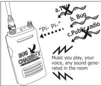
8. When bug picks up the discriminating tone sent by BC-EX, the bug also send it back again to the air. BC-EX receives the raido signal which containing the discriminating tone, it judges the signal is from bug and automatically changes to audio mode and you can hear what you received.
