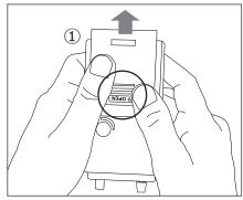
Remove the lid of battery box first. Hold the body like the picture on the left. Press the part marked with a circle and slide it toward the direction of arrow (①).
