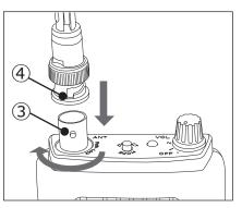
3.Attach antenna to the antenna termninal. Now, Bug Chaser EX (BC-EX) is ready.
