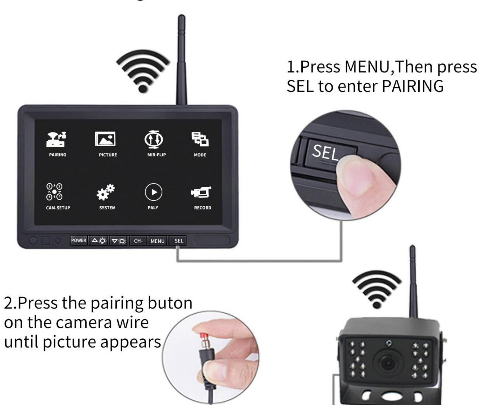
Note: the system has been paired successfully at the factory, and if you need to rematch, refer to steps 1 and 2 above.
