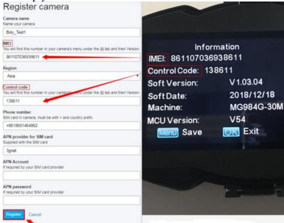
2.4 Please insert SIM card, SD card, external power or batteries. Move the switch to test, wait the camera register the operator, then press menu key to enter menu setting page.
